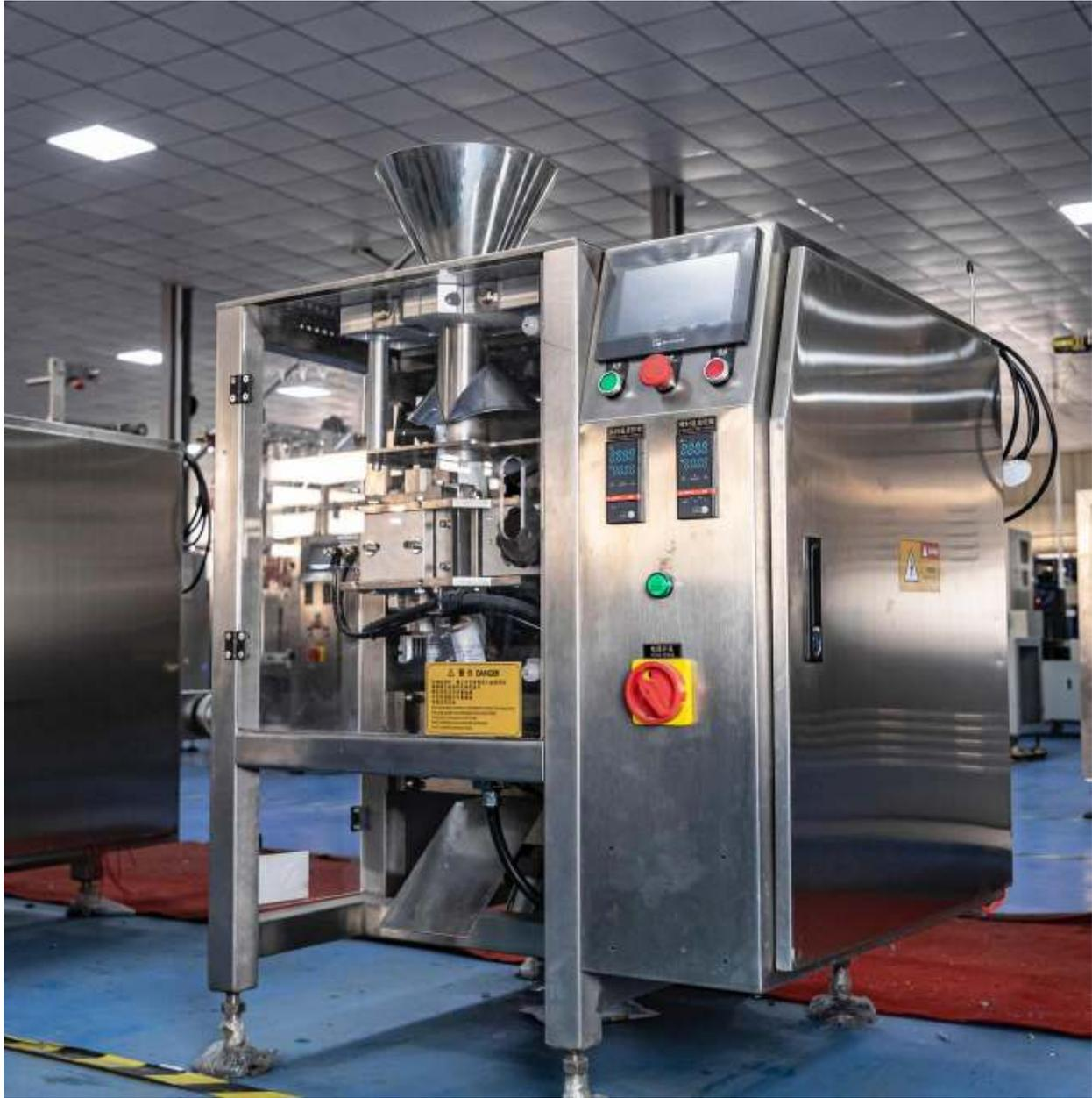
On the other hand, [vertical packaging machines](#) are designed to work with [powdery](#), granular, or liquid products in form. These items need to be packaged in a way that will ensure their stability and prevent them from leakage.
