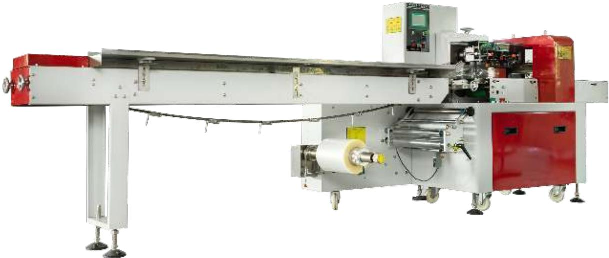
Horizontal packaging machine also called horizontal flow wrap machine, It is best to use horizontal packaging for single solid goods that can be readily handled, such as cereal bars, soaps, tiny toys, bakery products, and other similar items.
