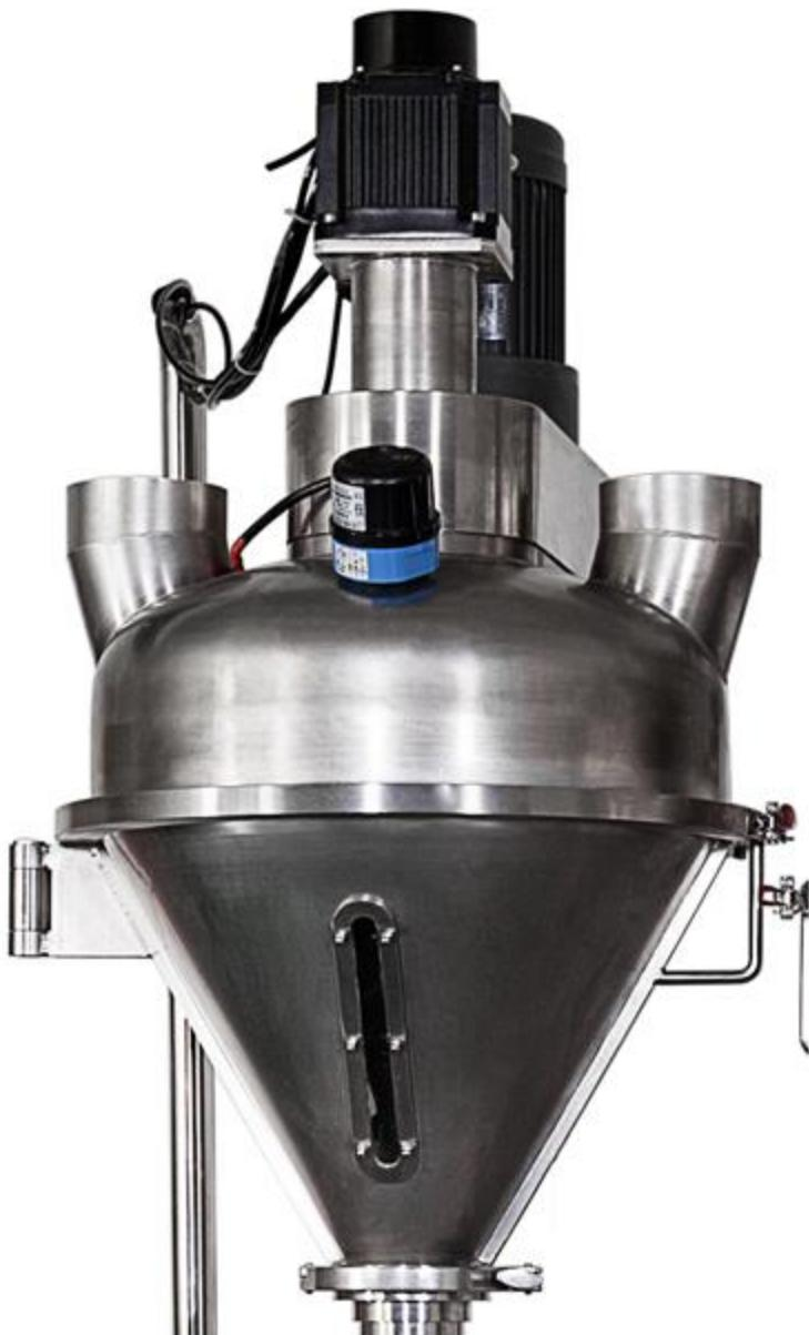
[Automated nitrogen filling](#) is possible because the machine is specifically developed for powder, ultrafine powder, and other materials; it is capable of completing all of the necessary tasks.
